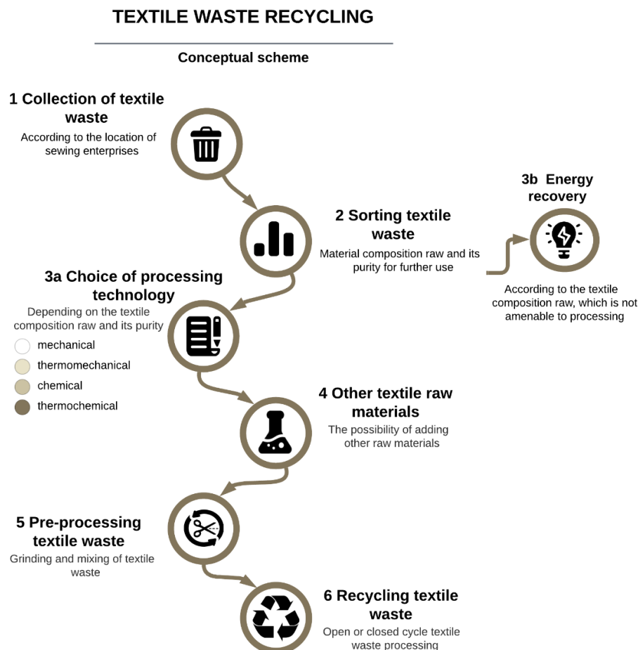
Fig. 1. Conceptual scheme of recycling textile waste
